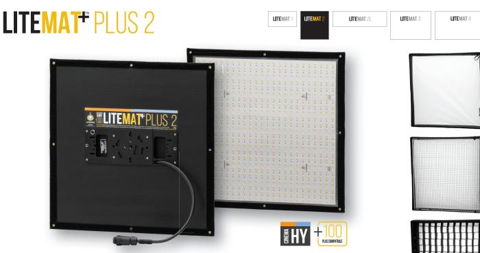
The LiteMat+ Plus 2 is based on two "tiled" light engines, each measuring 9.5 in. x 19 in. (240 mm x 480 mm). The head unit features 1152 new CineMitter LEDs and is covered by a thin, clear polycarbonate layer and bordered entirely with Velcro® "loop" fastener. Mounting is provided with a Kino Flo®-compatible, removable gimbal mount. The "soft-through-pixelization" method allows the LiteMat+ Plus 2 to achieve surprisingly bright light levels.
